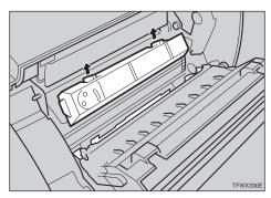
2 Insert a new waste toner bottle at the rear of the photoconductor unit.
